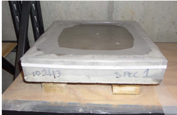
Figure 2.10. Ponding Chloride Test Specimen with 5% Sodium Chloride Solution
