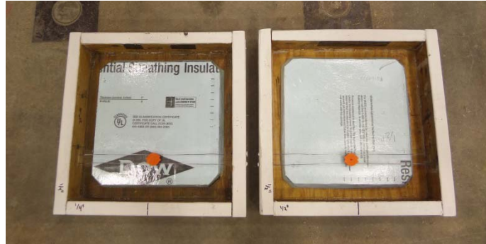
a) Molds and RFID Sensors' Installation Detail
